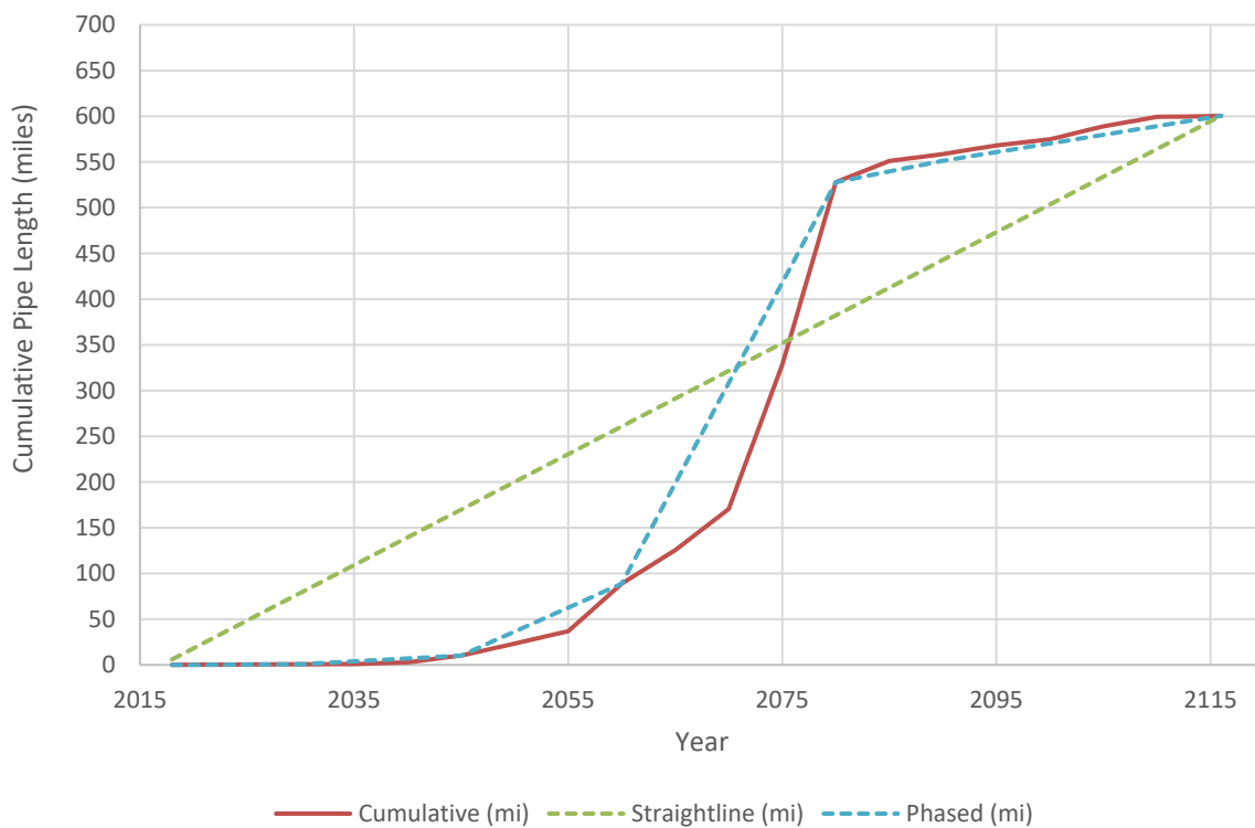
Figure 7-3. Representative Pipeline Replacement Strategies
