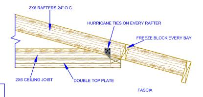
MIN PITCH OF ROOF FOR SHINGLES
