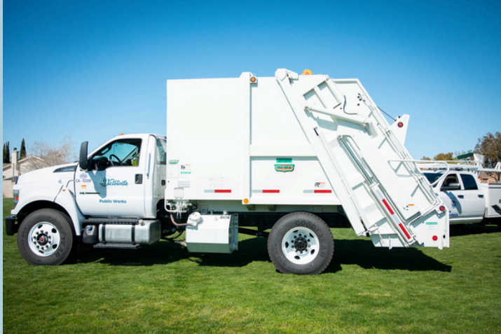
Public Works Compacting Rear Loader
